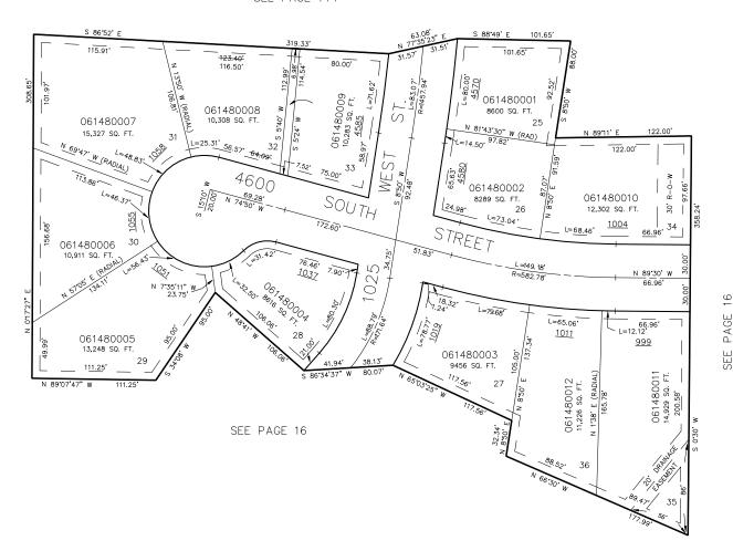
7' UTILITY & DRAINAGE EASEMENTS EACH SIDE OF PROPERTY LINES AS INDICATED BY DASHED LINES EXCEPT AS OTHERWISE SHOWN.
